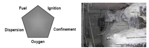
Many insurance companies insist on strict housekeeping, sanitation, and preventive maintenance atm insured elevators. Grain, broken kernels, and grain dust accumulate in the leg boots and should be cleaned out periodically. Some elevators install easily removable doors on leg boot side panels for quick, easy cleanout.
